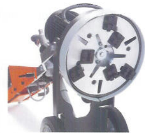
Single grinding plate with multiple diamond tool distribution positions.
